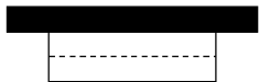
Counter-top with storage above Standard counter-tops are 24 inches deep. Standard top cupboard storage is 12 inches deep.
